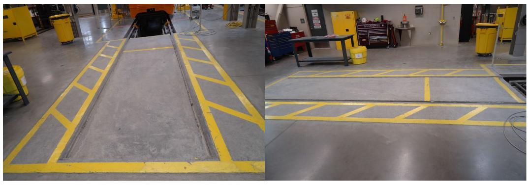
Spare truck storage was mapped to occupy the space at the head of Bay-2, but the space was delineated to also allow for movement around the truck for prep and servicing as well as to avoid blocking the pit stairs.
