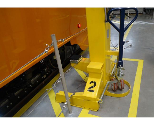
Vehicle power jacks have specific storage areas that also offer a defined range for safe deployment allowing the streetcar placement flexibility when spotted within the service bay.
