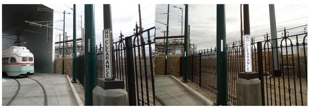
There are several areas in the yard apron that have no clearance when a streetcar is present and moving through the area. No clearance signs with 3M Hi-Reflectivity coating light up brightly with even the smallest amount of light. All OCS support poles are numbered and fed into a GIS mapping system. This makes it for easy locating and OCS maintenance.
