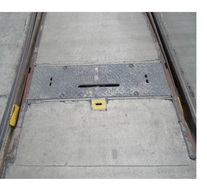
Out in the yard apron are voestalpine Nortrak CSV-34 Embedded Manual Switch Machine with the switch points coated in reflective yellow paint. This allows for easy switch point position identification in low light conditions.
