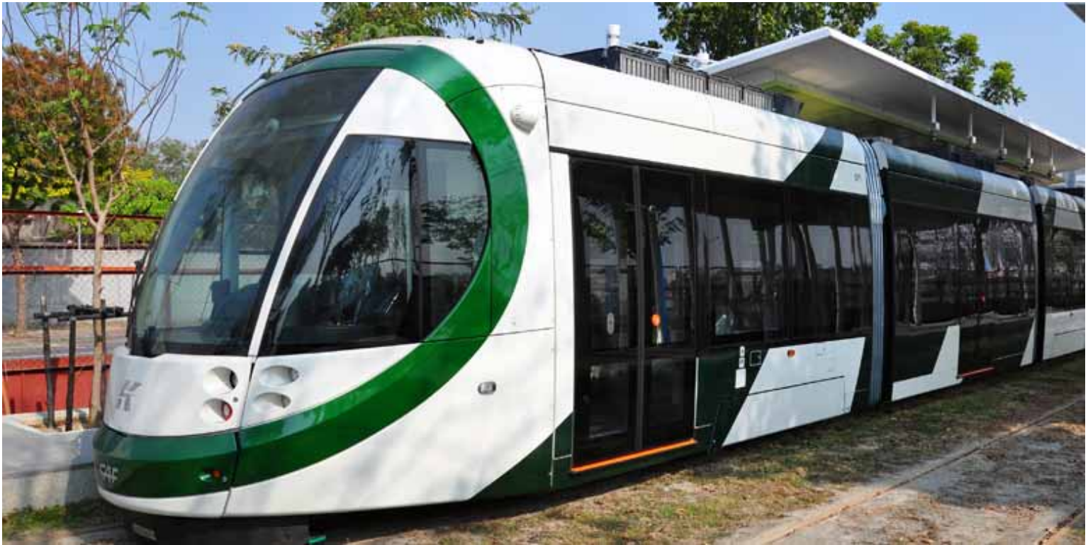
Kaohsiung, Taiwan - 8.2 km catenary-free line, using onboard energy storage with recharging at each station
