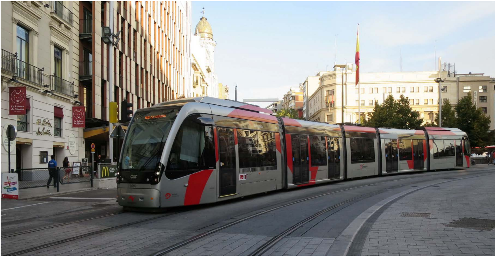
Zaragoza, Spain- 2 km off-wire segment using onboard energy storage, opened 2013
