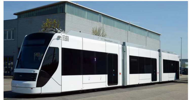
Doha, Qatar - 11.5 km catenary-free line, using onboard energy storage with recharging at each station. Opening 2016
