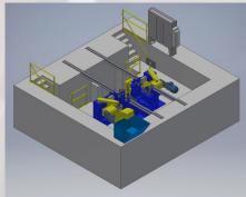
M2: Underfloor Machine For Light Rail Vehicles (20 Ton Max Axle Load)
